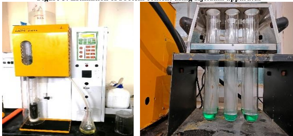
Figure 3: Estimation of Protein content using Kjeldahl apparatus
