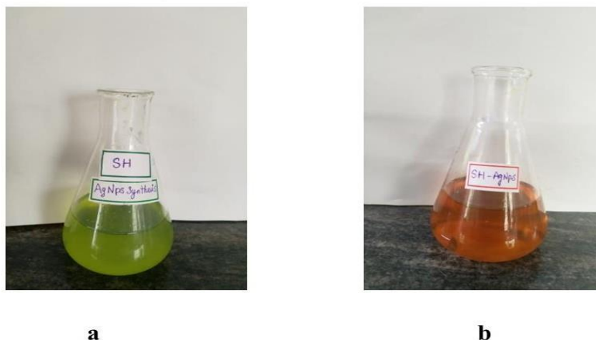
Figure 3.1: Visible observation; A) silver nitrate with whole plant extract of S. hamata , B) Synthesised silver nanoparticles from the whole plant extract of S. hamata
