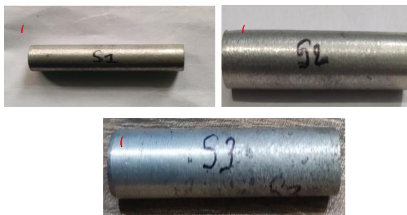
Figure 1. (a) AZ91D, (b) AZ91D/1.5 wt. % B 4 C/0.2 wt. % MWCNT, (c) AZ91D/1.5 wt. % B 4 C/0.4 wt. % MWCNT wear samples.
