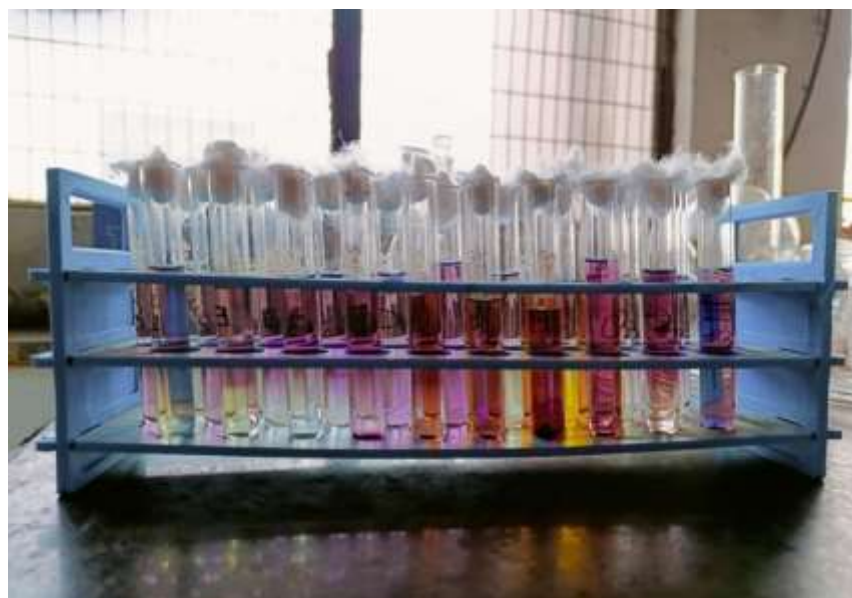
Fig 3: Picture representing the solution mixtures containing D.P.P.H. and synthesized compound
