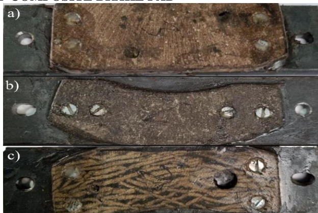
Figure 3: Brake pads with a) Coconut fibres b) Agave fibres c) Sisal fibres
