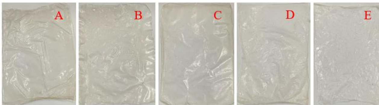
Figure 1. Composite bioplastics (a) EL0, (b) EL20, (c) EL40, (d) EL60, (e) EL80.
